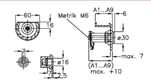
Door + frame thickness = 52-60 Measure type = A8
